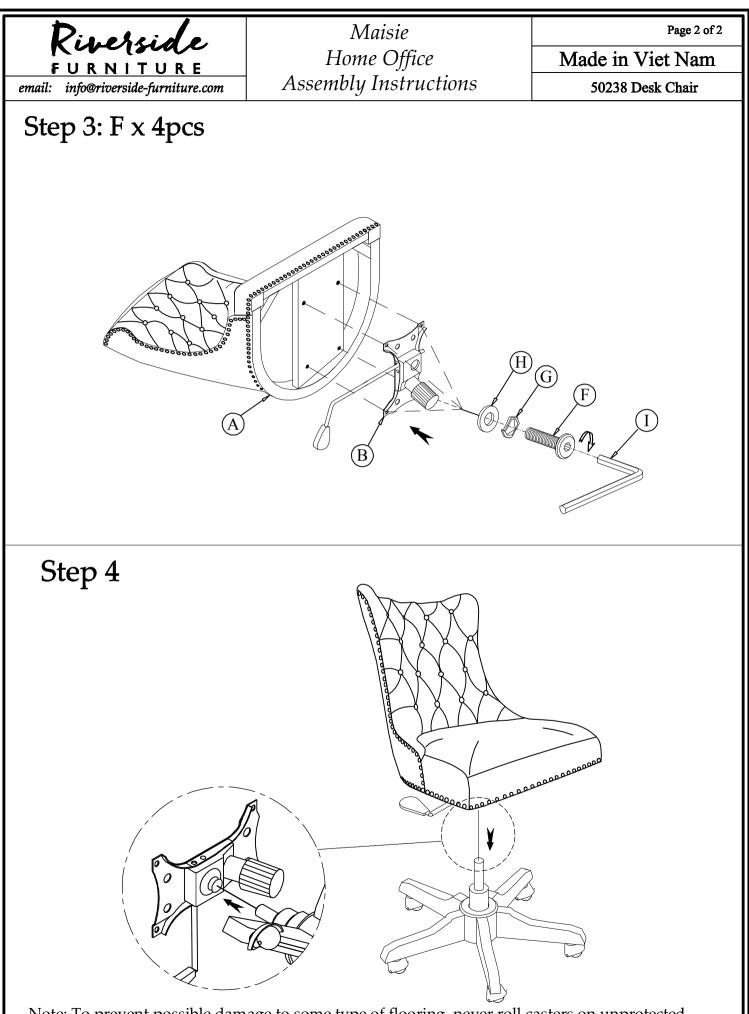
Note: To prevent possible damage to some type of flooring, never roll casters on unprotected hardwood or vinyl flooring. The lift mechanism is in a locked position for shipping. To unlock, pull straight out on the handle, and then the lift cylinder can be activated by lifting the handle.
